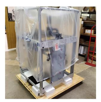
Before arrival, establish an appropriate space for the Gigabot<sup>®</sup> X to be located during operation. Gigabot<sup>®</sup> X requires access to a dedicated 15A circuit, and should be plugged into an uninterrupted power supply or a surge protector. A climate-controlled environment is recommended, but not necessary. Gigabot<sup>®</sup> X operates best at a temperature of 16°C (60° F) to 29°C (85°F) and at a humidity of 0%RH to 80%RH non-condensing.
