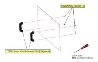
If your Gigabot<sup>®</sup> X includes an enclosure, you will need to attach [11229] Panel Handles to the Hood Panel Front, both Hood Panel Sides, and Front Panel Top prior to use. Fasten using [10231] M4 x 12 FHCS and 2.5mm Allen Wrench.
