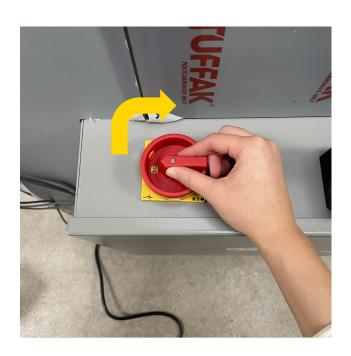
If you are looking at the back of your Gigabot<sup>®</sup> X, the power switch is located on top of the electrical box. It is a large red switch; rotate it clockwise to turn it on.
