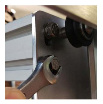
Use the 8mm combination wrench to gradually tighten the [10540] M5 x 12 HHCS at each quadrant. Periodically use the tool setter to check the bed level, since tightening the hardware on the rails may slightly move them.
