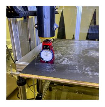
Using the Viki LCD controller, move the bed down 101.3mm, or the height of your tool setter minus 0.3mm. To do this, navigate to the "Prepare" menu, then "Move Axis," then "Move Z," then "Move 10mm," and finally turn the dial clockwise until it reaches 100mm. Navigate back to "Move 0.1mm" and move the bed down until it reaches 101.3mm.
