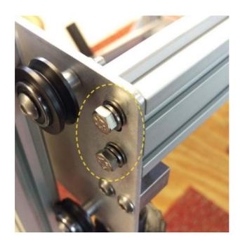
To level the bed, identify the quadrants that need adjusting and use the 8mm combination wrench to loosen the  $2 [10540] \,\text{M5} \, \text{x} \, 12$  HHCS that fasten the bed side plate to the bed cross rails. These need to be loose enough so the ends of the rails can move vertically in the slots of the side plates.
