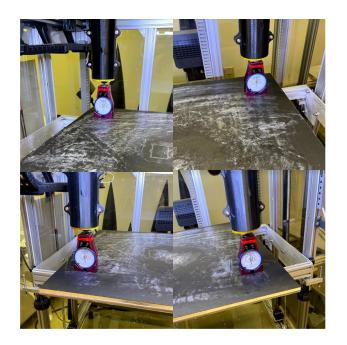
If all the quadrants have a value other than zero, then the Z height must be adjusted (otherwise, skip to B10). To do this, move the tool setter to the back left quadrant. Use an 8mm combination wrench to adjust the [10245] M5 x 70 HHCS on the upper Z limit switch leveling block (on the right side of the machine). Turning counterclockwise when viewed from above will increase the Z height, and clockwise will decrease the Z height.
