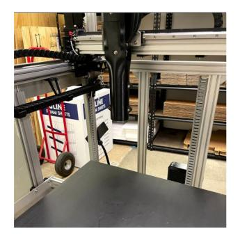
Push the extruder back until the nozzle is past the back edge of the bed. If the motors are engaged and the extruder doesn't move, use the Viki to disable the steppers. To do this, press the dial to reach the menus, scroll clockwise to select and click "Prepare", then scroll and press the dial to select "Disable Steppers".
