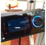
Using the Viki LCD controller, move the bed down 150mm. Press the button to see the main menu, then select "Prepare," scroll down to "Move Axis," then "Move 1mm," then "Move Z," and finally turn the wheel clockwise until it reaches 150mm.
