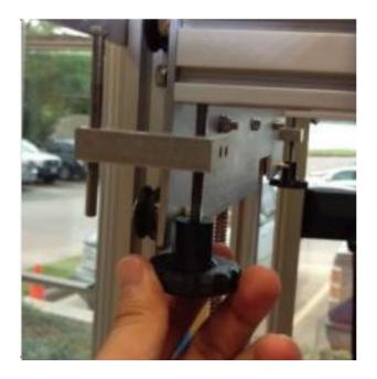
When viewed from below, turning the knob clockwise will raise that corner. Turn the leveling knob to raise the bed until the nozzle is close but not touching the shim stock. This gap is needed because when raising the other corners of the bed, this corner will also raise slightly. Repeat this process at all corners of the bed.
