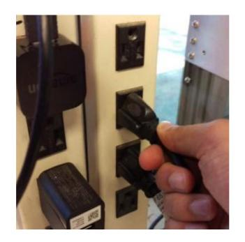
Insert the plug end of the power cable into an outlet.
