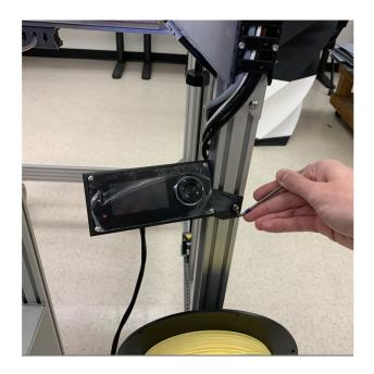
Locate the Viki at the back of the Gigabot<sup>®</sup> 3+ near the electrical box and remove all packaging from the Viki. With a 4mm Allen wrench, unscrew the three screw in the back upright rail and use the screws to attach the Viki to the rail.
