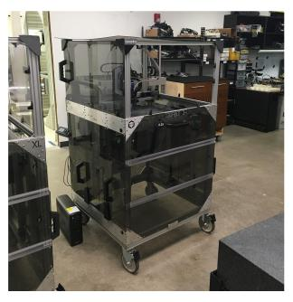
Before arrival, establish an appropriate space for the Gigabot<sup>®</sup> 3+ to be located during operation. Gigabot<sup>®</sup> 3+ requires access to a dedicated 110 VAC 15A circuit, and it should be plugged into an uninterrupted power supply or a surge protector. A climate-controlled environment is recommended, but not necessary.
