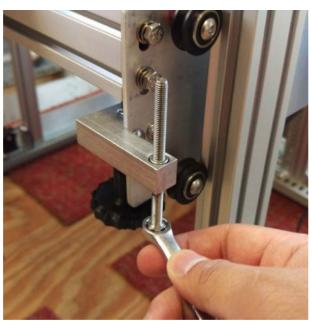
Adjust the leveling knobs until there is about a 1/8" gap (3mm) between the top of the rail and the top of the side plate at each corner. A ruler or a shim can be used to measure this distance. Similarly, users can opt to turn the leveling knob to push the rail up until it is flush with the side plate, and then lower it 4 full revolutions.
