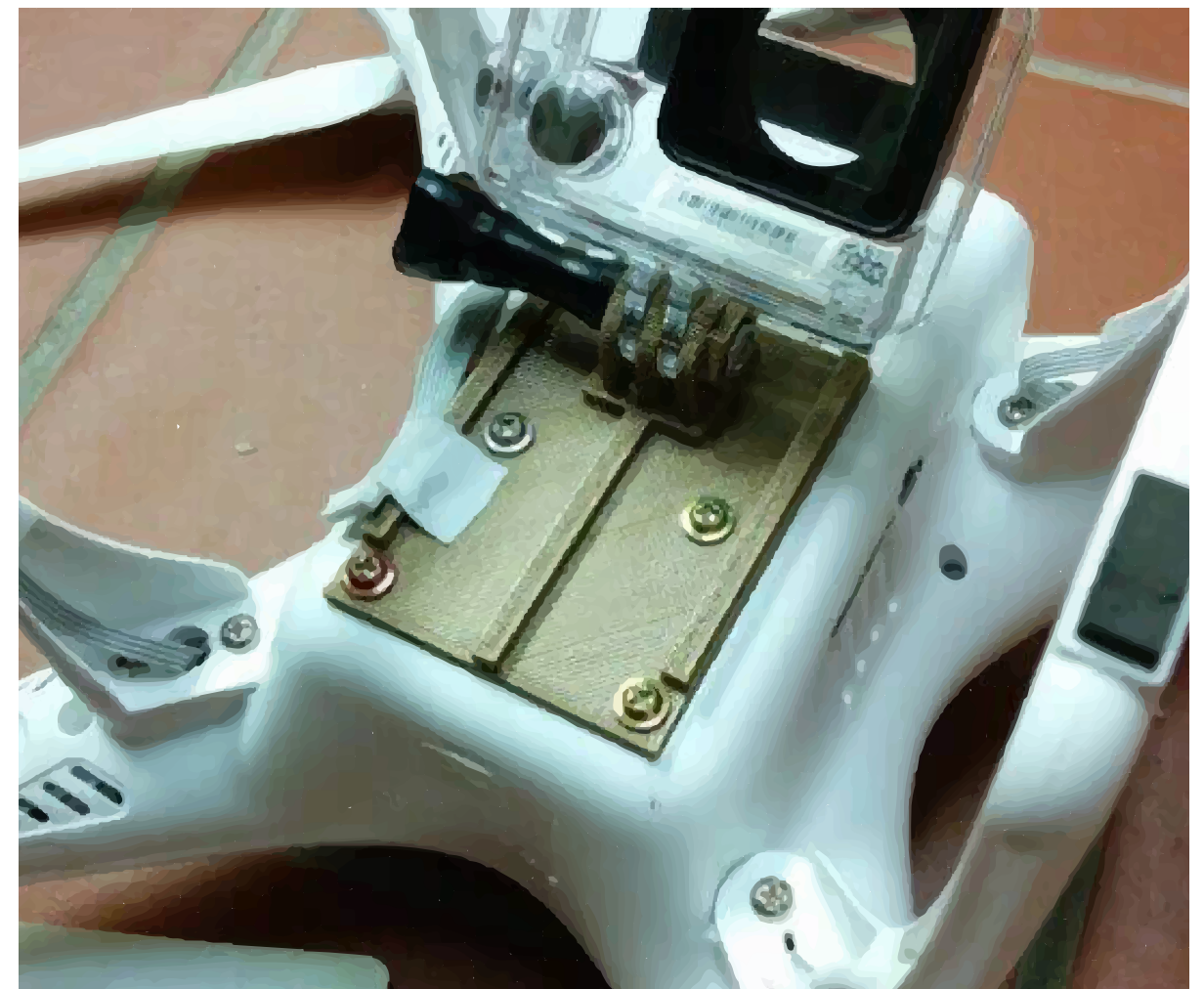
Pictured above: A 3D printed UAV camera mount Source: All3DP [13]
