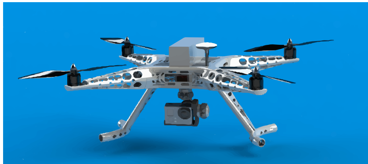
Pictured above: A rendering of a PLA UAV frame printed using SLS Source: Sculpteo [12]
